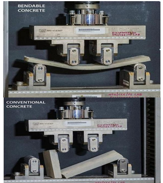
Concrete tablet testing Image courtesy NTU
