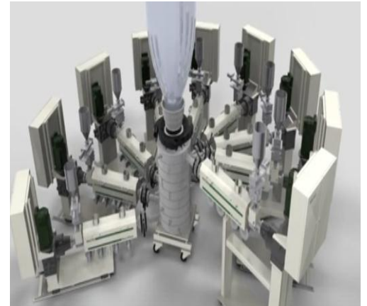
Multilayer blown film extrusion process
