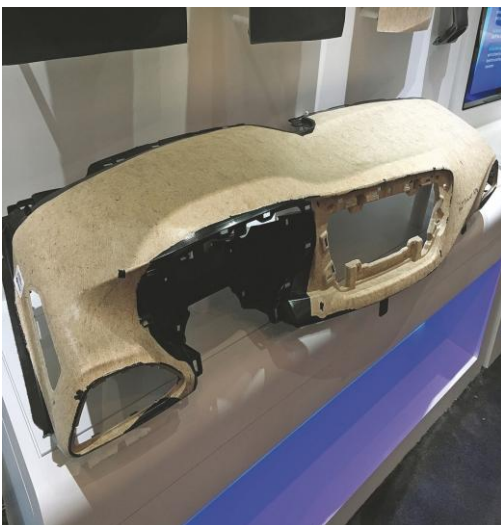
Car interior part made with compression hybrid molding
